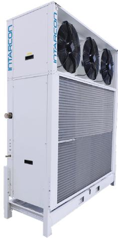
Vertical-mounted evaporating units designed for freezing tunnels, built in galvanised steel structure and bodywork with thermosetting polyester coating.
