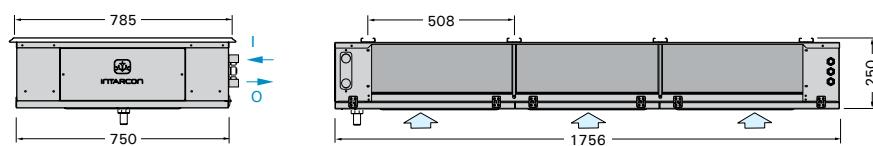
Nominal conditions are related to 12 °C cold room temperature and operation with propylene glycol in 20% volume concentration for 0 °C / 5 °C inlet/outlet temperature.
