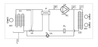
COMPRESSOR MV: MOTOR FAN EV: EVAPORATOR CD: CONDENSER
