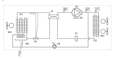
CP: COMPRESSOR MV: MOTOR FAN EV: EVAPORATOR CD: CONDENSER
