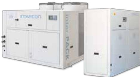
**intarPACK** refrigeration plants are packaged air-cooled, axial and centrifugal, direct expansion plants with hermetic reciprocating or scroll compressor/s, from 4 to 60 HP for evaporating temperature range from -45 °C to +5 °C.
