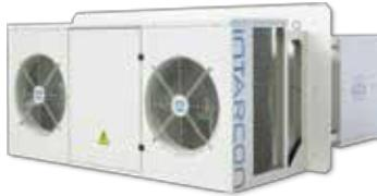
**superblock** series are industrial refrigeration monoblock units for large size cold rooms up to 2 000 m<sup>3</sup>, featuring hermetic reciprocating or scroll compressors for temperature range from -25 °C to +15 °C.
